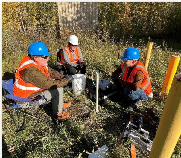
Groundwater sampling (source: EPA 2024)
